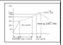
Put the connector on the P.C. Board and expose them to the reflow oven for 2 times
